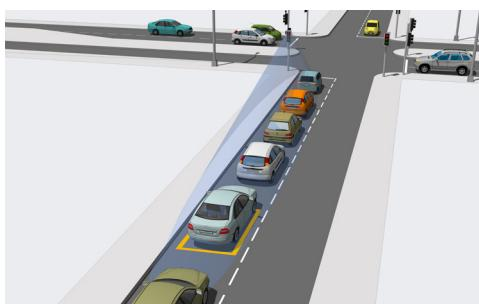
The AGD318's accurate virtual-loop technology, with speed discrimination & stationary detection can emulate two inductive-loops up to a range of up to 150 metres, or lane-specific detection up to 40 metres with one AGD318 per lane. In traffic control applications, the AGD318 tracks up to 12 targets and 'reports' when virtual-loops are triggered. The AGD318 can make loops 'smart' as well - for example, to prioritise buses over cars at bus-gates.
